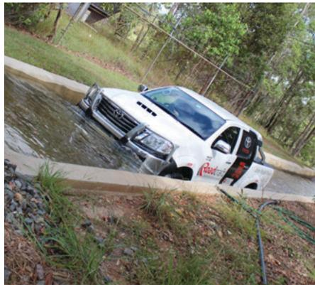
**Purpose-built 4WD water crossing** and traction-seeking pad
